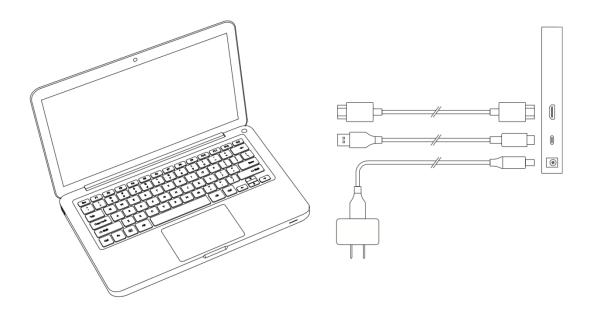
2. USB-C connection (Only full-featured USB-C port): Connect the pen display to your computer with a USB-C cable. Then connect the power jack to the adapter connected to the wall outlet.
