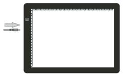
3) Plug the power adapter into the power input jack of the light pad, then press the touch switch button briefly to turn the light pad on; press the touch switch button briefly again to turn the light pad off.
