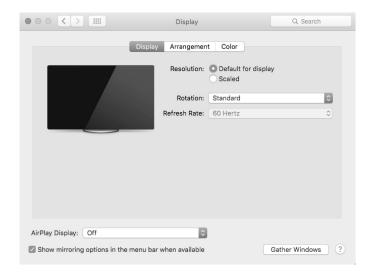
(6). In the "Arrangement" tab, disable "Mirror Display" and set the Artist 10S to "Monitor 2." Set the tablet's resolution to 1280x800 or 1280x720 (depending on monitor 1's aspect ratio).
